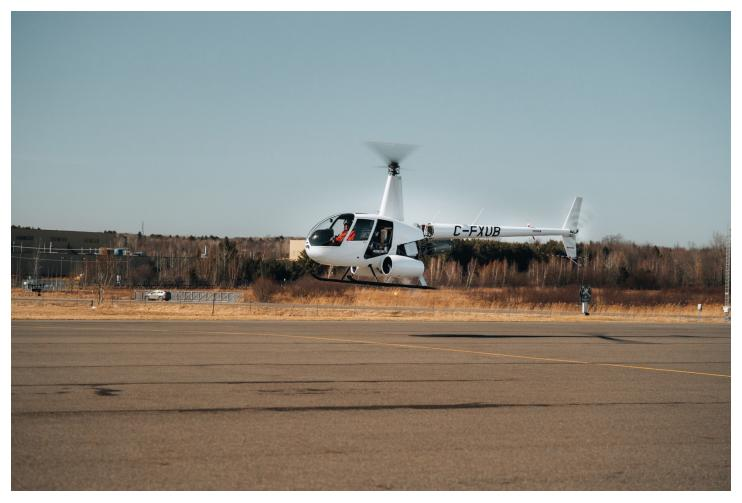
Test pilot Ric Webb of Unither Bioélectronique performs a hover flight in the company's experimental hydrogen-powered Robinson R-44 Raven II helicopter at Roland-Désourdy Airport in Bromont, Québec, March 27, 2025.
