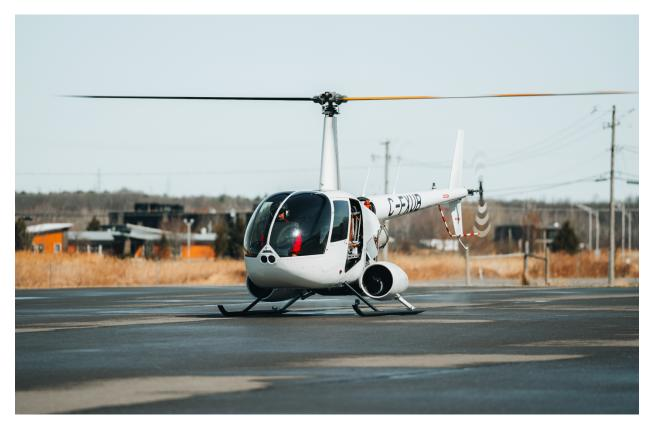
Ric Webb of Unither Bioélectronique performs pre-flight checks in the company's experimental hydrogen-powered Robinson R-44 Raven II helicopter at Roland-Désourdy Airport in Bromont, Québec, March 27, 2025.
