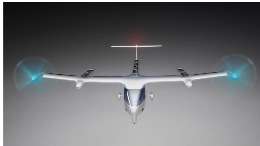
Quiet: many eVTOL aircraft may fly in a wing borne configuration most of the time, resulting in virtually silent overflight.
