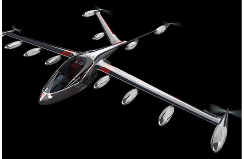
Figure 7 - Artist's Rendering of Joby Aviation 4 Seat Electric Vertical Take Off and Landing Air Taxi Prototype
