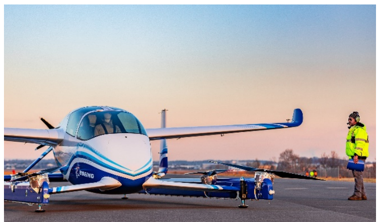
Figure 4 - Four Passenger All-Electric Boeing Design Utilizing Eight Rotors
