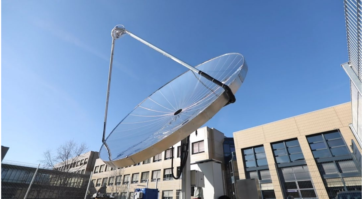
Figure 12: EPFL's PEC Parabolic Dish[39]
