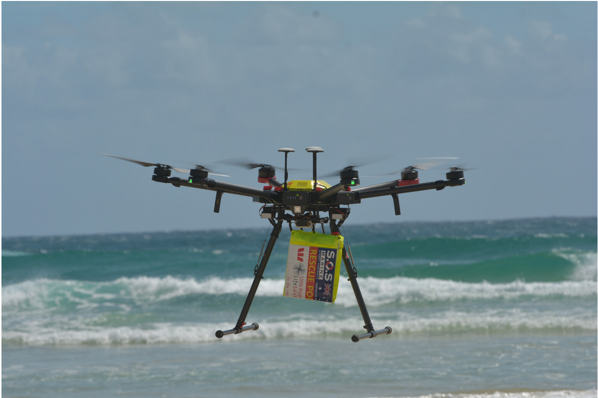
FIGURE 1.1 Westpac Little Ripper Saver drone with inflatable lifesaving device known as a “rescue pod” that was dropped to swimmers in high surf in New South Wales, Australia, January 2018. SOURCE: Leanne St. George & Associates Pty Ltd.
