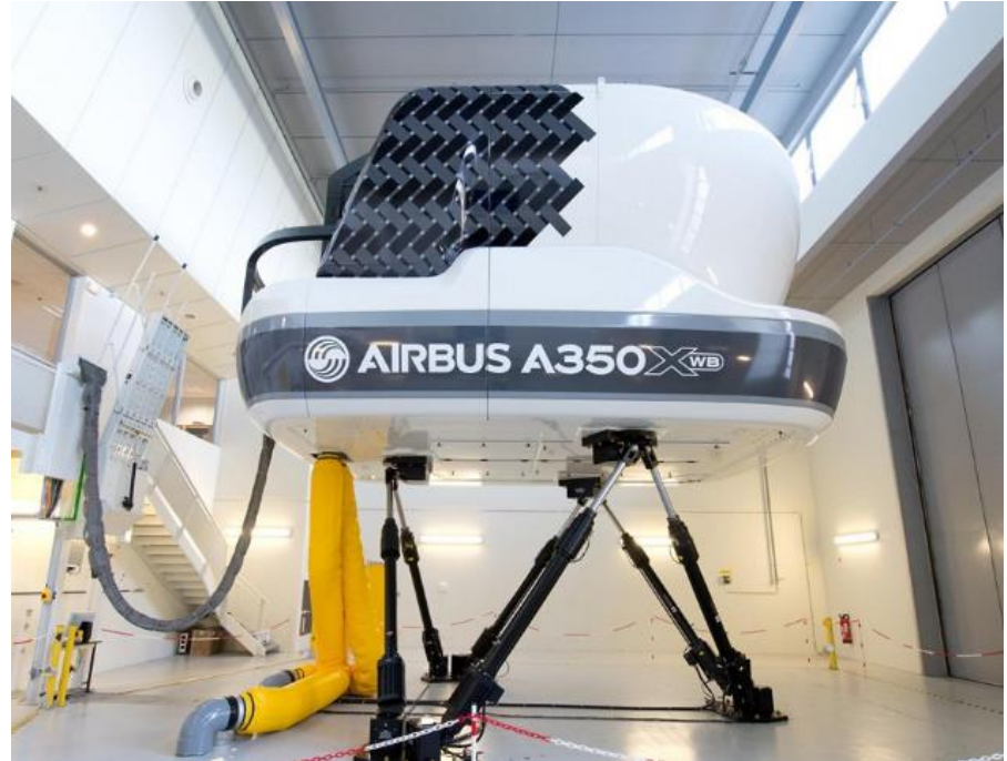
Figure 30. A350XWB Full-flight Simulator (FFS) located in the Airbus Flight Training Center in Toulouse
