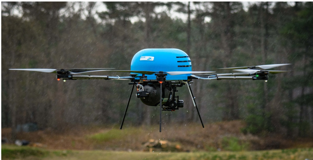
Figure 8 BFD's Hydrogen Fuel Cell Hex-rotor. Water is the only emission.
