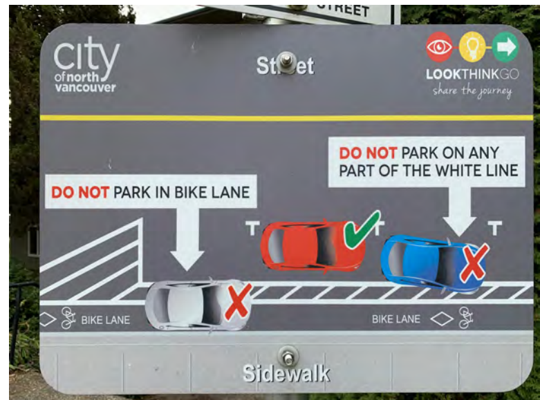
Signage indicating where to park adjacent to a parking protected bicycle lane, City of North Vancouver, B.C.
