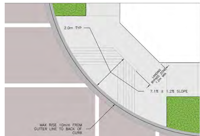
FIGURE G-82 // COMBINED CURB RAMP
