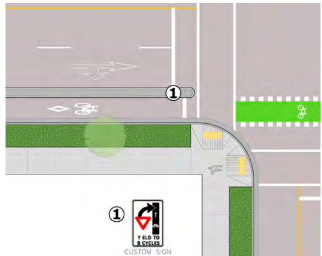
FIGURE G-93 // PROTECTED BICYCLE LANE ADJACENT TO COMBINED RIGHT THROUGH TURN LANE
