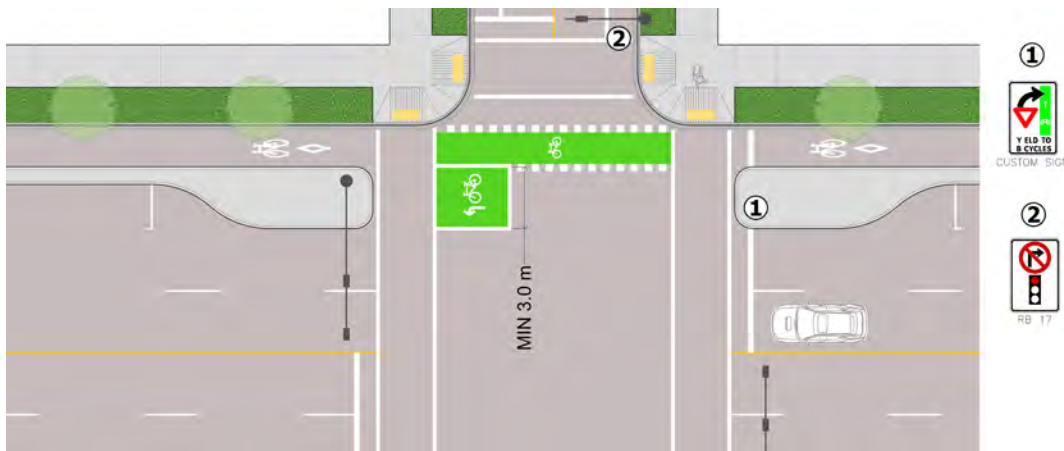
FIGURE G-105 // PROTECTED BICYCLE LANE WITH TWO-STAGE LEFT TURN BOX
