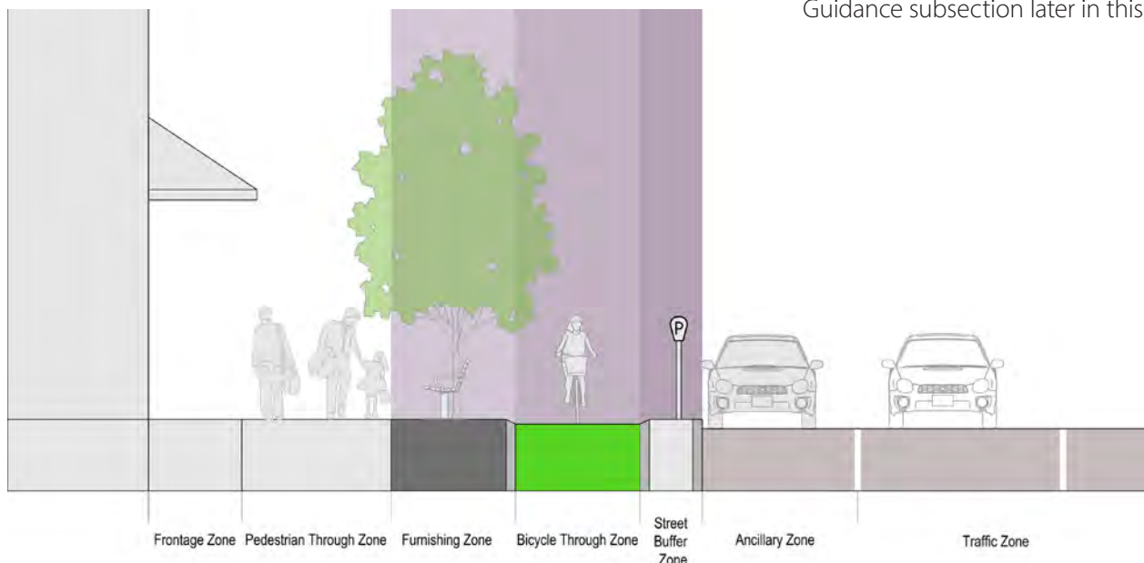
FIGURE D-37 // PROTECTED BICYCLE LANE ZONES
