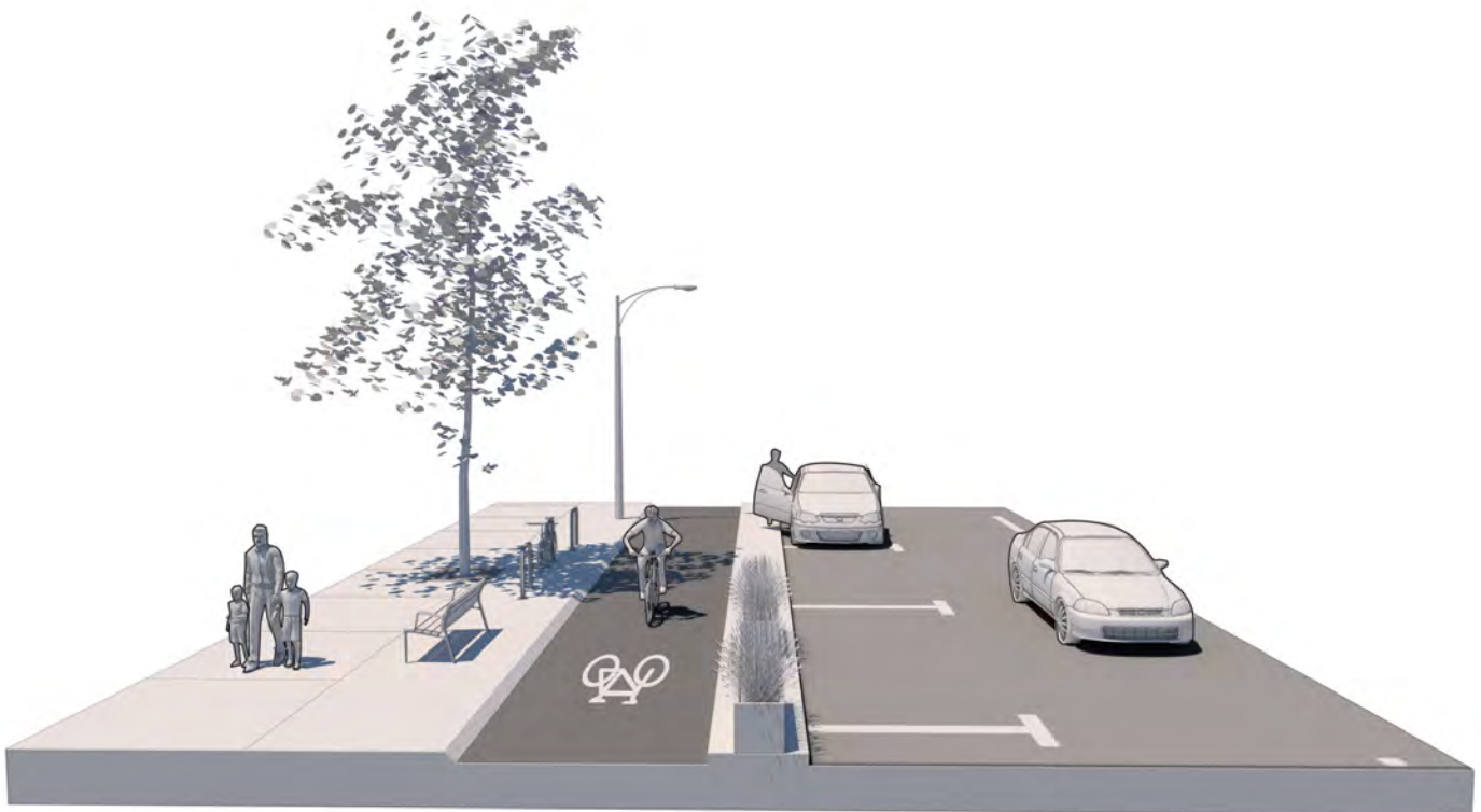
FIGURE D-46 // STREET LEVEL PROTECTED BICYCLE LANES
