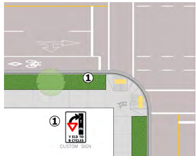
FIGURE G-94 // PAINTED BICYCLE LANE ADJACENT TO COMBINED RIGHT THROUGH TURN LANE
