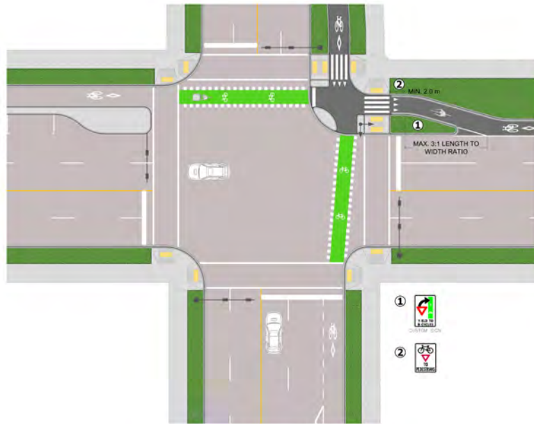
FIGURE G-113 // BICYCLE LANE TRANSITIONING TO PROTECTED CORNER
