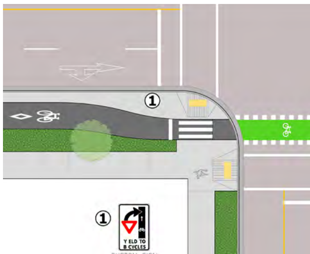
FIGURE G-92 // BEND-OUT PROTECTED BICYCLE LANE
