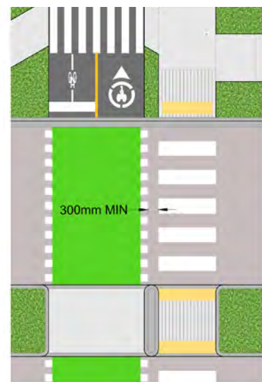
FIGURE G-126 // SEPARATED CROSSING PAVEMENT MARKINGS
