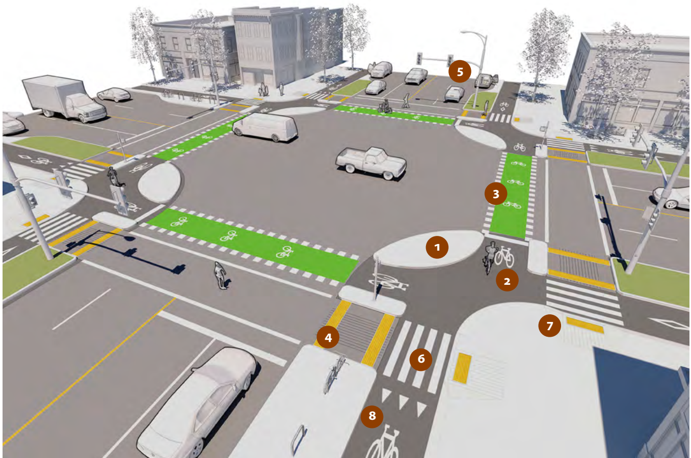
FIGURE G-90 // PROTECTED INTERSECTION KEY FEATURES
