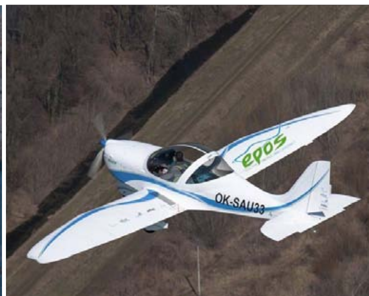
The SportStar EPOS was one of the first electric UL built in series production. It used a REB 90 Engine (80 kW), MGM COMPRO HBC 400400 Controller (photo below) and LiPo 80 Ah battery pack (360 V).
