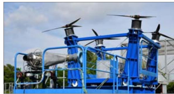
Safran's HEPS hybrid system has been put into ground test since last June up to 100kw power output (photo credit: Safran)
