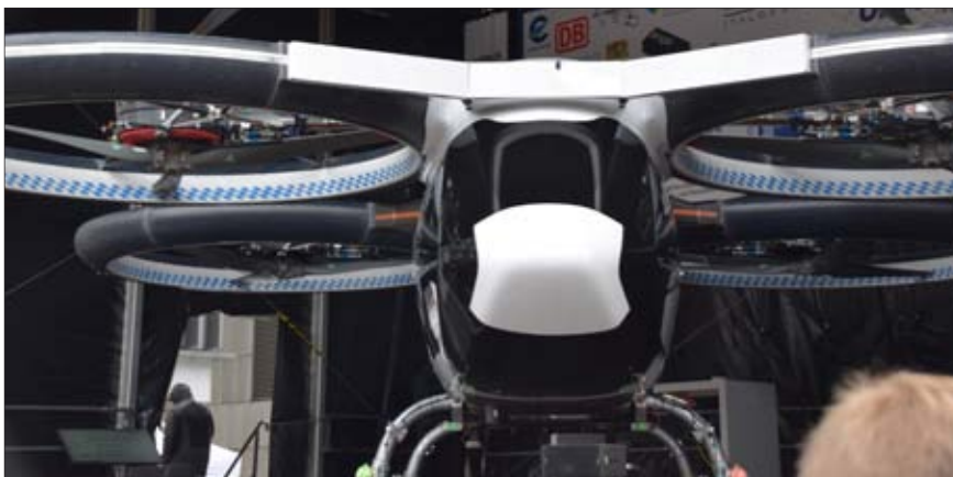
The upper rotor is outside the duct and inclined towards the front of the vehicle
