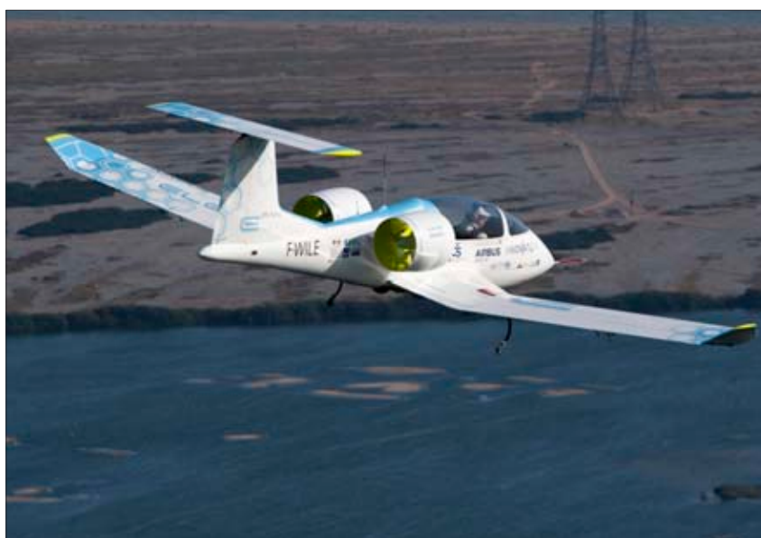
Airbus E-Fan with four RET 60 (25 kW) engines and one REG 30 (7 kW) engine for the wheel gear. Flying time is around 40 minutes.
