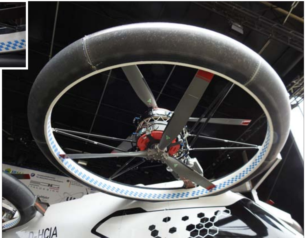
Details of the coaxial electric motor structure. Note: the Bavaria color decoration in the inner ring of the duct.
